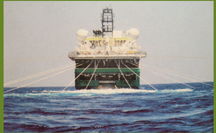
Recording equipment being towed behind a survey ship
